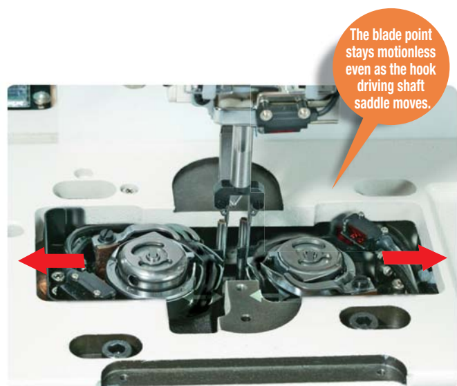
Image of the hook driving shaft saddle in motion
